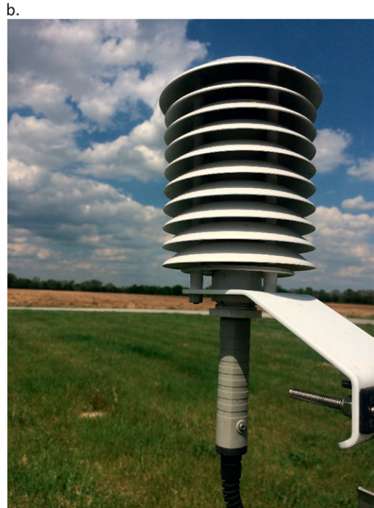
FIG. 4. (a) Aspirated radiation shield and (b) Gill radiation shield (naturally ventilated).
