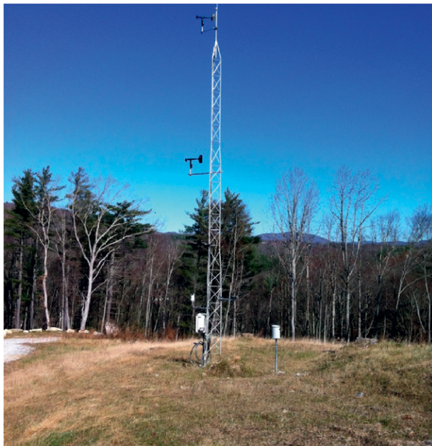
FIG. 7. A mesonet station in North Carolina with nearby obstructions (trees).
