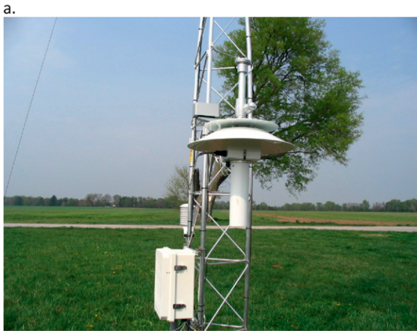
FIG. 4. (a) Aspirated radiation shield and (b) Gill radiation shield (naturally ventilated).
